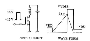
$$\begin{aligned} R_G &= 25~\Omega \\ V_{DD} &= 90~V,~L = 4.8~mH \end{aligned} \qquad E_{AS} &= \frac{1}{2} \cdot L \cdot I^2 \cdot \left( \frac{BV_{DSS}}{BV_{DSS} - V_{DD}} \right) \end{aligned}$$
